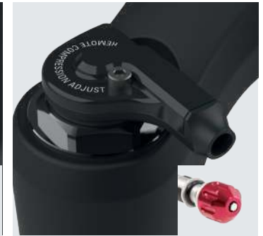
R-3CR-PCS Remote Lockout with 3 positions of compression (firm setting, medium setting and open setting) with low speed rebound adjust along with PCS system.
