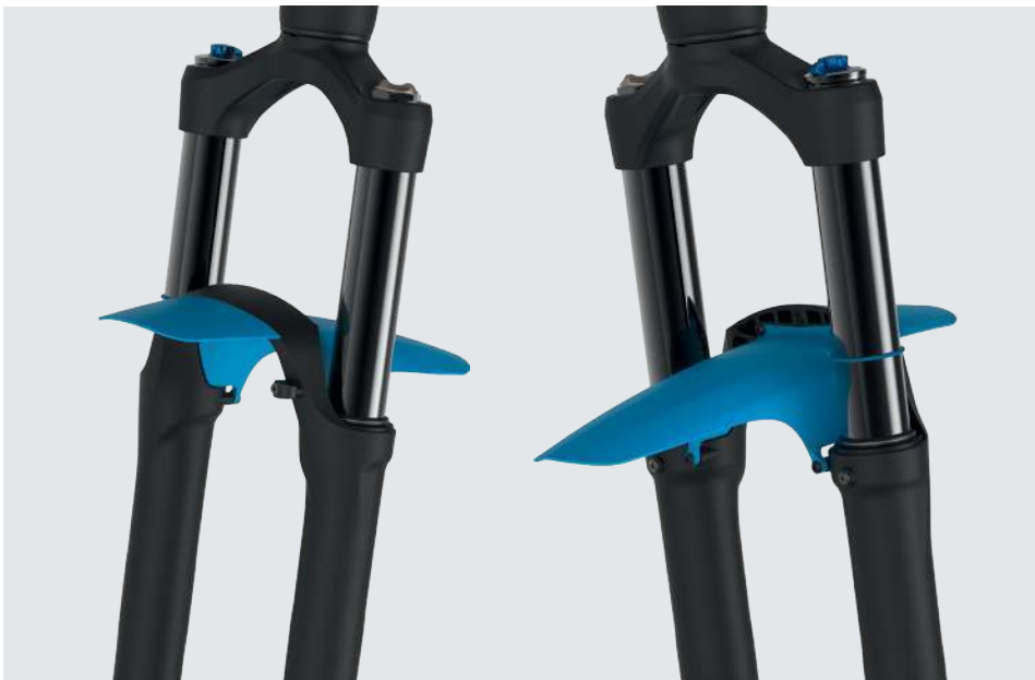
SHORT FENDER MOUNT Detachable integrated short fender
